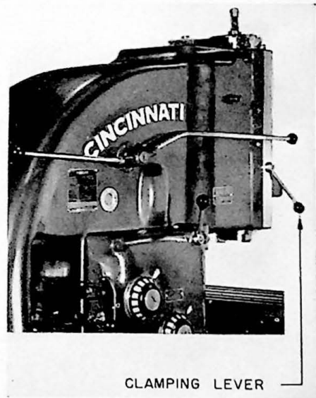
Figure 12 Left Hand Side of Vertical Head, Showing Clamping Lever
