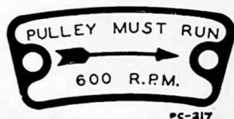
Figure 5 Main Drive Pulley Must Rotate in This Direction Viewed From Rear of Machine
