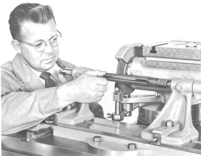
"Tange-Bar" Taper Setting Device assures accurate angles when grinding straight fluted taper reamers.
