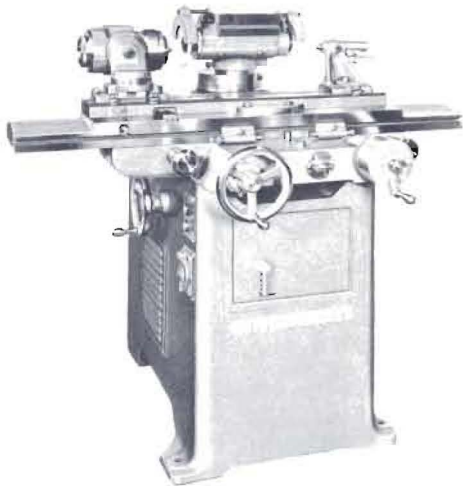
Duplicate Controls . . . located at front, right or left-hand end of table; rear right or left-hand side of column; for convenience of operating machine from any position.
