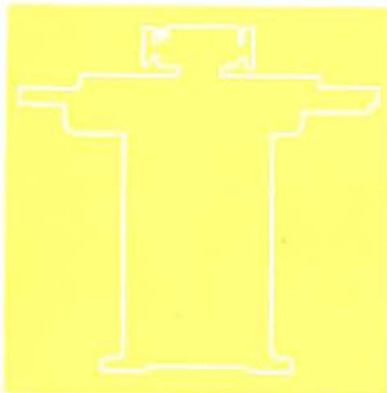
Slenderized Box Type Bed with Fixed Height Table . . . maintains accuracy of table traverse and enables operator to get closer to machine to observe actual grinding.
