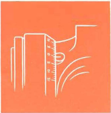
Clearance Setting Dials On Universal Workhead and Left-Hand Tailstock . . . legibly graduated for convenient and accurate setting of predetermined clearance angles.
