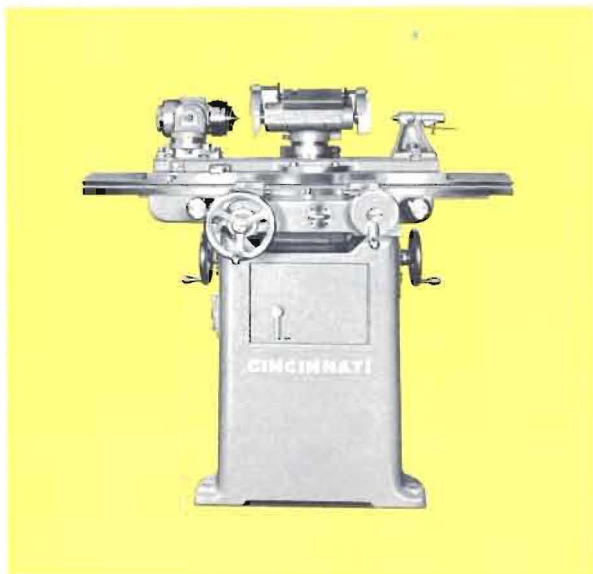
Slenderized bed enables the operator to get in close and be comfortable whether seated or standing.
