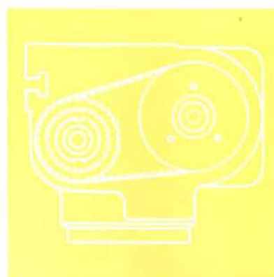
Positive Spindle Drive . . . power grip belt provides positive drive from the instantly reversible motor to the grinding wheel spindle.
