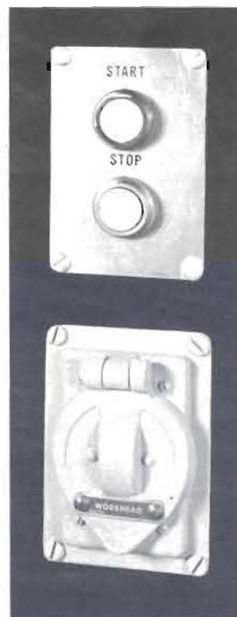
Built-in push buttons are located on both the right (shown below) and left (shown at left) sides of the base, easily within the reach of the operator.
