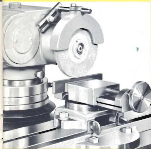
Improved surface finish on surface grinding operations are obtained by having the grinding wheel positioned directly over the work.
