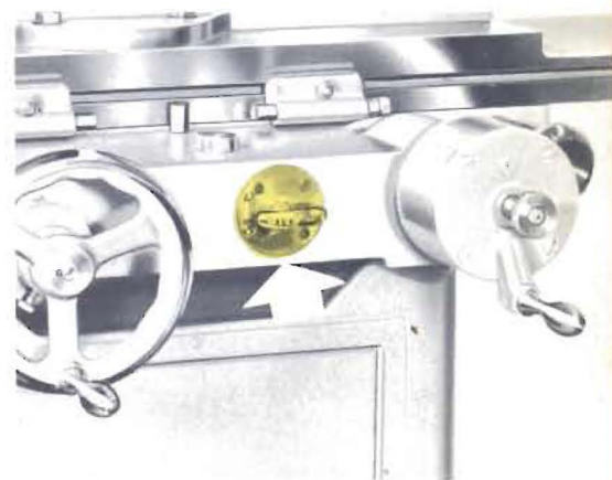
Oil-shot pressure lubrication system reduces daily service requirements.
