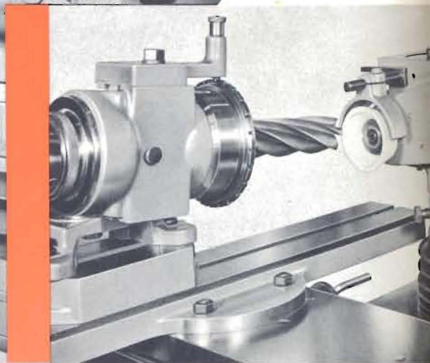
Universal workhead and Indexing Attachment aid in sharpening end of extra long end mill.
