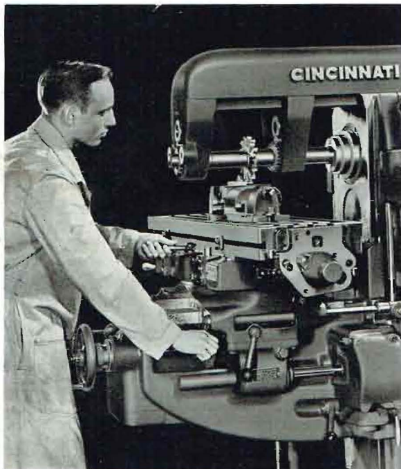
RECTANGULAR OVERARM WITH PILOT WHEEL CONTROL Pilot wheel control cuts down the effort of moving the overarm when changing cutters or arbors. It's convenient, too, for the overarm clamping nuts are near the pilot wheel, at a normal height to apply leverage on the wrench.
