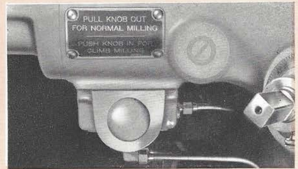
Control knob for engaging and disengaging automatic backlash eliminator.
