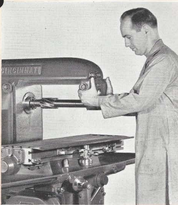
Arbor supports are easily removed and replaced on the overarm.
