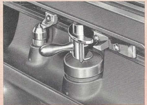
Four-position hand table control lever. Action of table in various lever positions indicated below.
