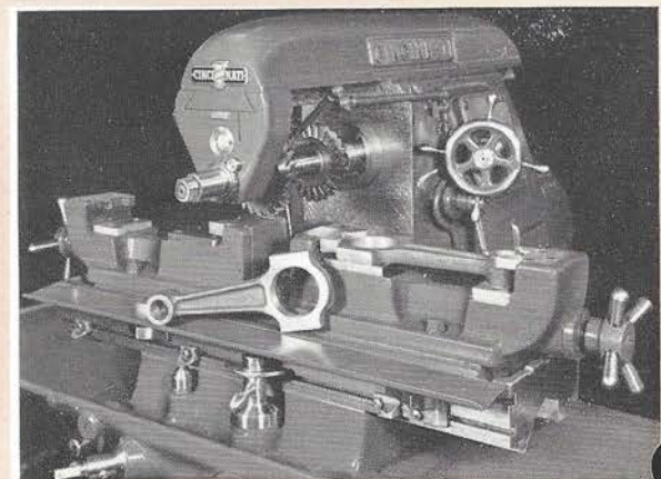
Both automatic spindle stop and automatic backlash eliminator are useful features for this job.
