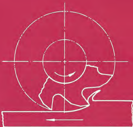
Conventional, or Up Milling . . .
