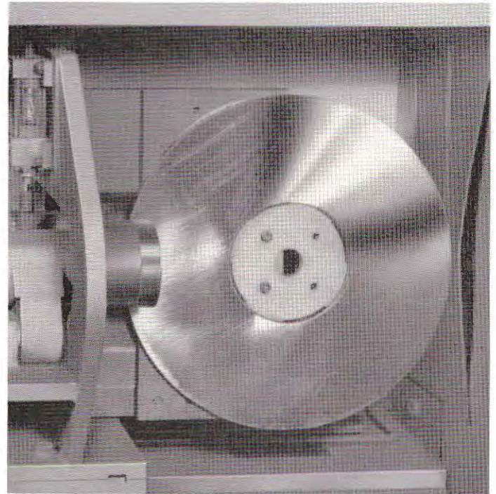
Hydraulically operated reciprocating fixture, with rotating work holder, arranged for handling disk plates.
