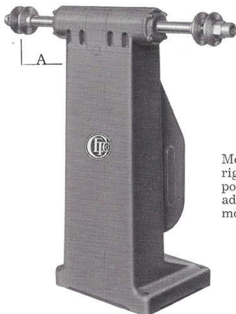
With open type spindle extensions. Two ball bearings. (Front view.)
