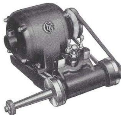
Illustrating Open Type Internal Grinding Head Mounted in Place of External Grinding Head
