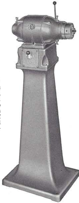
← WITH No. 2 TAPER SOCKET Furnished in speeds for direct drive, 1750 or 3400 R.P.M. For gear drive, 90 to 3400 R.P.M. Switch enclosed in base of motor. 4" Universal 3 jaw chuck on ap- plication.
