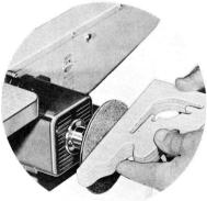
DISC SANDER For shaping small pieces and trueing-up uneven surfaces. Sanding discs are mounted on rubber backing pad.
