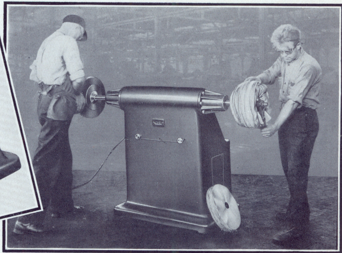
This application illustrates the versatility of this machine and the time saving that can be effected. It is not necessary to stop work on both spindles when a buff or wheel must be changed on one end only. Another advantage of paramount importance is the fact that jobs requiring different working speeds may be handled on the one machine at the same time.
