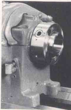
Right—Type L Long Taper Key Drive Spindle Nose.
