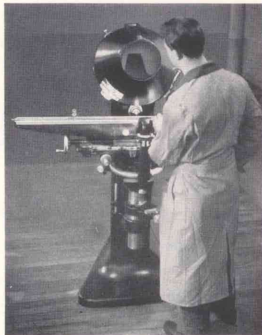
Fig. 2. Inspecting a Screw Thread with an Optical Comparator.
