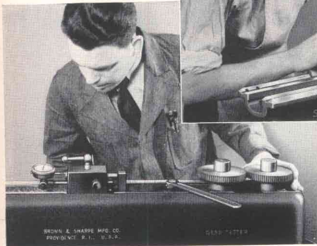
Fig. 6. Below—Testing Gears for Accuracy of Tooth Form, Pitch Diameter, and Concentricity
