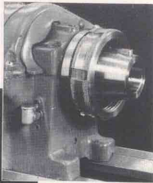
Right—Type L Long Taper Key Drive Spindle Nose.
