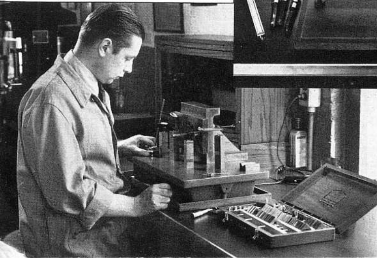
Fig. 2. Below—Checking the Accuracy of a Fixture with Precision Gauge Blocks Accurate to Five-Millionths of an Inch. Extreme Accuracy necessary for perfect interchangeability of parts is assured by frequent testing of jigs and fixtures
