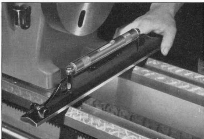
Fig. 17. A precision level must be used for leveling the lathe.
