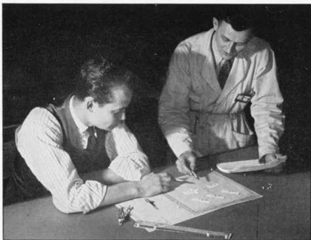
Fig. 4. Planning the arrangement of shop equipment with floor plan and cardboard cutouts.
