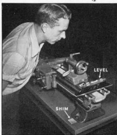
Fig. 18. Bench lathes are leveled by placing shims between the lathe and the bench.
