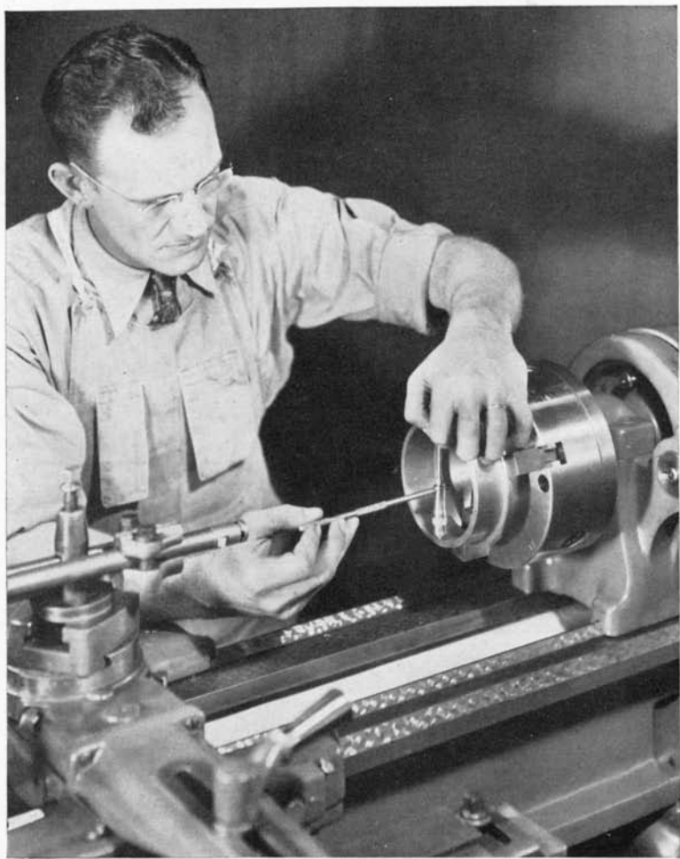
Fig. 1. To do accurate work, a lathe must be properly installed and leveled.
