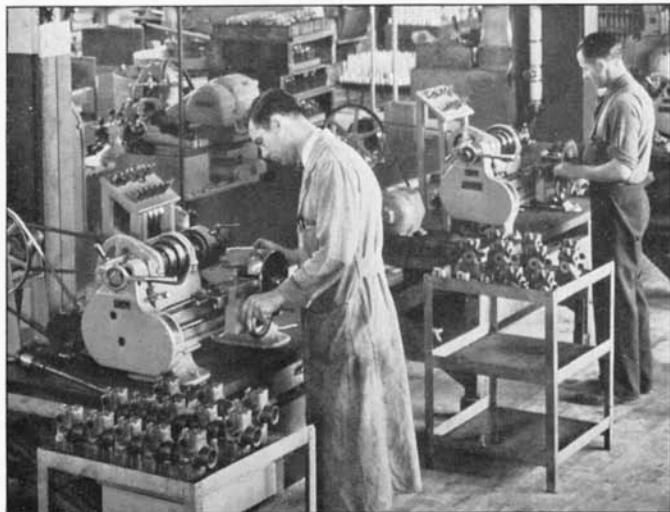
Fig. 11. When the lathe is used on production operations space must be provided for stacking unfinished and finished work.
