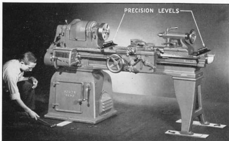
Fig. 15. The lathe must be carefully leveled, using shims between the legs and the floor.
