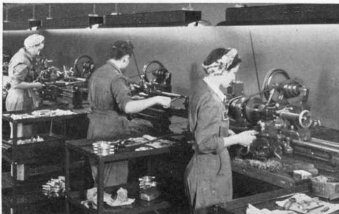
Fig. 6. Good general illumination is provided by fluorescent lights in deep reflectors mounted well above the line of vision.
