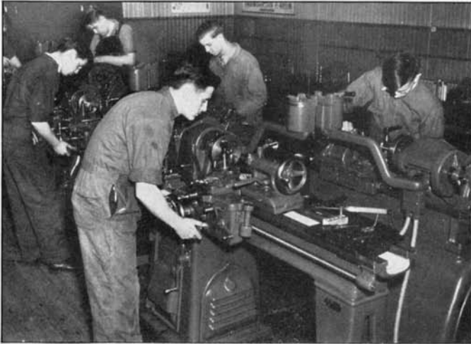
Fig. 13. Lathes placed back to back to save floor space.
