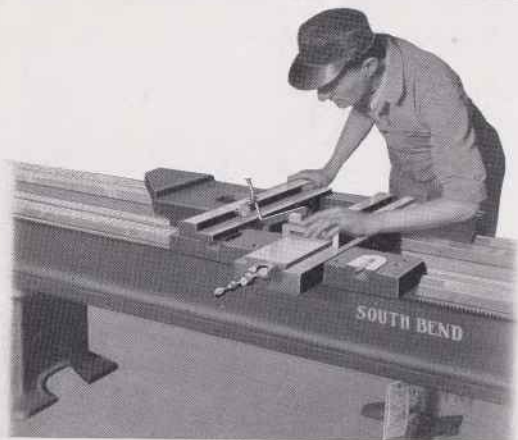
Testing Cross Side of Saddle
