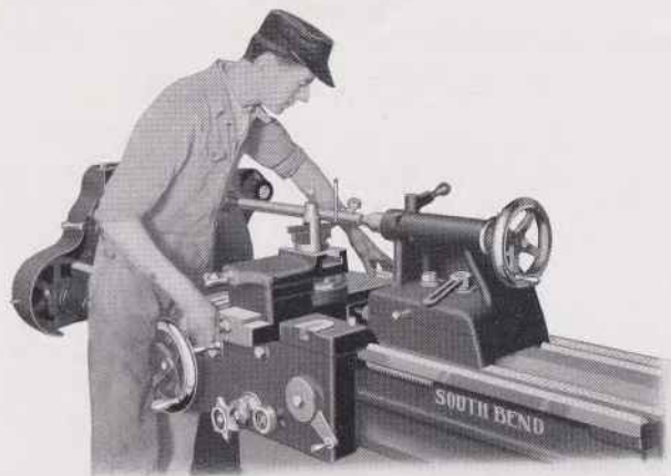
Testing Alignment of Head and Tail Stock
