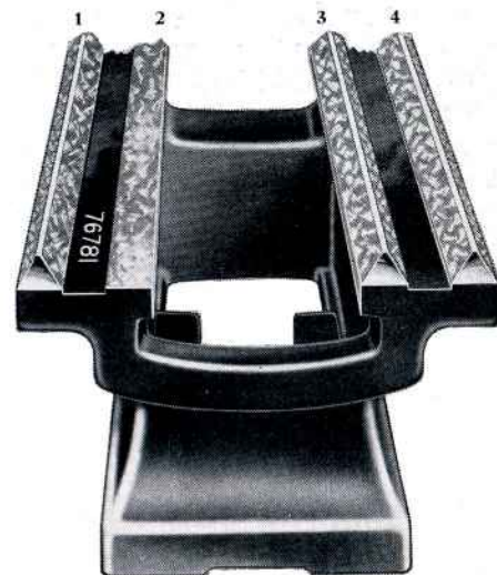
Fig. 20. End View of Lathe Bed Showing Prismatic V-Ways
