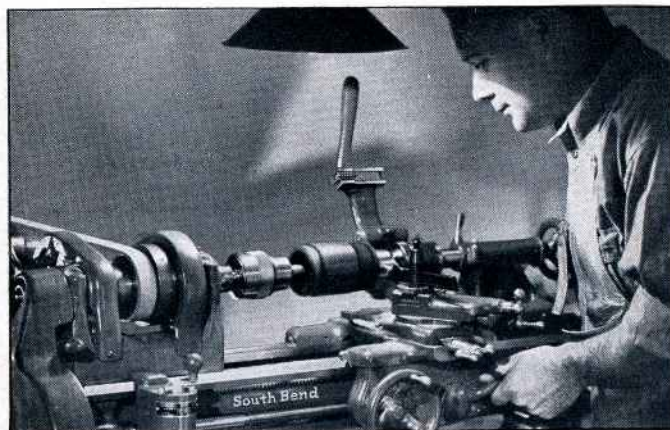
Fig. 327. Truing and Undercutting an Armature Commutator in the Lathe
