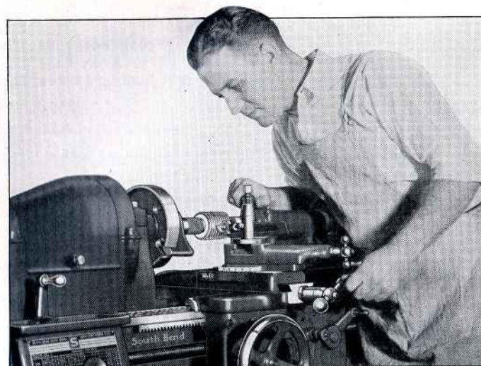
Fig. 204. Cutting Screw Threads in the Lathe
