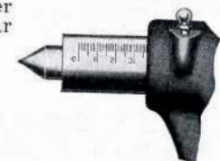
Fig. 314. Metric Graduations on Tailstock Spindle
