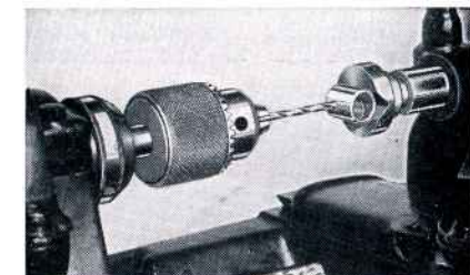
Fig. 188. Drilling an Oil Hole in a Bushing with Crotch Center in Tailstock
