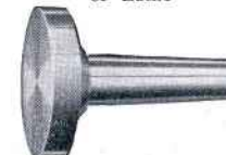
Fig. 187. (Right) Crotch Center for Use in Tailstock of Lathe
