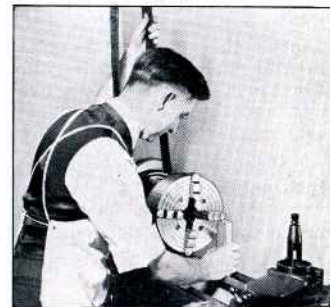
Fig. 156. Removing a Chuck from Lathe Spindle
