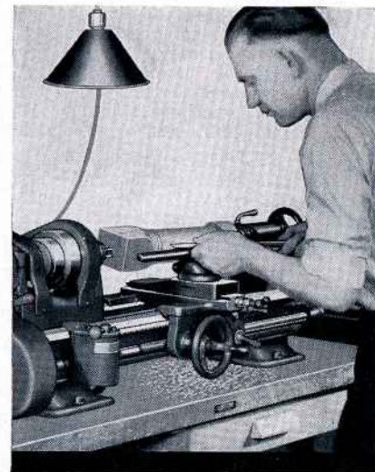
Fig. 307. Wood Turning in a Metal Working Lathe
