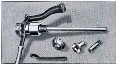
Fig. 169. Handlever Type Draw-in Collet Chuck Attachment
