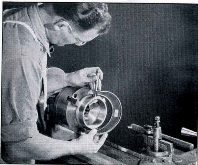
Fig. 111. Using an Outside Micrometer Caliper Measuring the Diameter of Work in the Lathe
