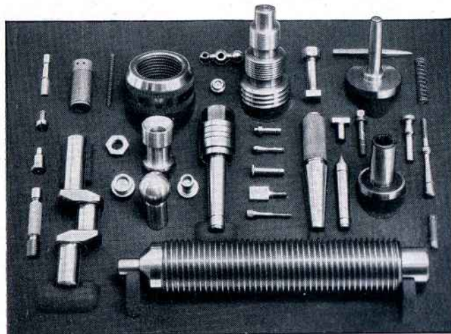
Fig. 340. Metal Parts Machined Entirely on a 9-in. Swing Back-Geared Screw Cutting Precision Lathe
