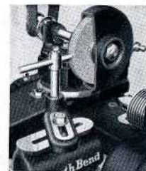
Fig. 317. Truing a Grinding Wheel with a Diamond Dresser
