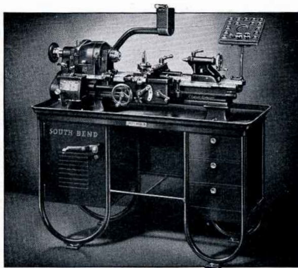
Fig. 323. A 10-in. Swing Bench Lathe with 1-in. Collet Capacity
