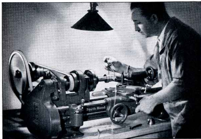
Fig. 339. Metal Turning on a Small Back-Geared Screw Cutting Lathe
