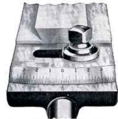
Fig. 182A. Graduations in Inches per Foot on Swivel Bar
