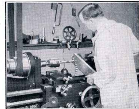
Fig. 186. Using the Lathe as a Drill Press
