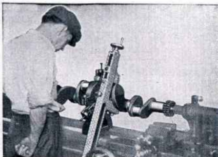
Fig. 336. Truing the Throw Bearings of a Crankshaft
