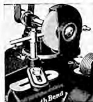
Grinding a Cutter in the Lathe
