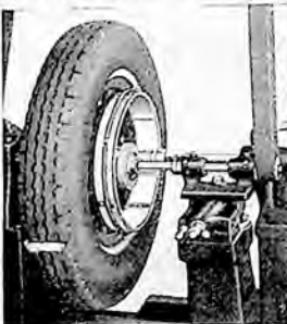
Grinding a Brake Drum on the Brake Drum Lathe
