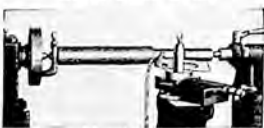
Making a Mandrel for Mounting Front or Rear Wheel
