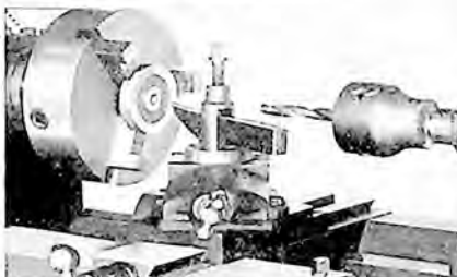
Drilling and Facing a Cast Iron Gear Blank Held in a Lathe Chuck. Drill Chuck Mounted in the Tail Spindle
