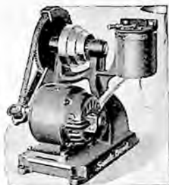
End View of Drive Unit Part of Gear Guard Removed to Show the Chain
