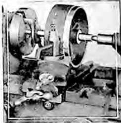
Machining a Cast Iron Pulley
