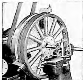
Boring a Wood Wheel for New Hub and Brake Drum
