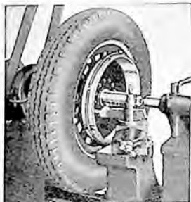
Truing a Four-Wheel Brake Drum, Making It Concentric with Axis of Hub
