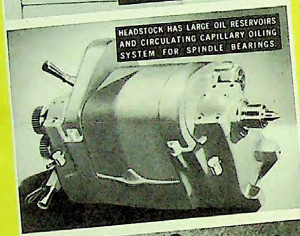
THREE-STEP CONE PULLEY HEADSTOCK, EACH STEP 3" wide
