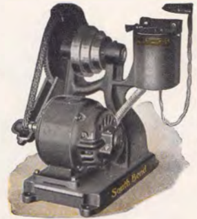
End View of Drive Unit Gear Guard Removed
