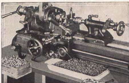
Hand Lever Type Draw-in Collet Chuck Forming and Cutting Off Duplicate Parts from Bar Stock
