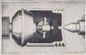
A Cross Section of a Piston on Adapter Ready for Machining
