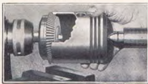
Reaming the Bevel Skirt of a Warped Piston so That It Will Fit True on the Adapter
