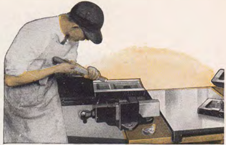
Hand Scraping Tailstock Base to Lathe Bed
