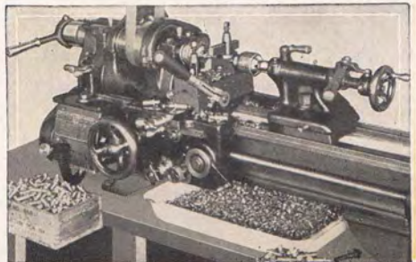
11-inch Lathe with Three Hand Lever-Type Attachments, Draw-in Chuck, Tailstock and Cross Slide
