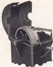
Cabinet Top Open Showing Drive Pulley
