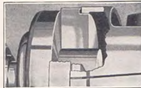
Close Up Showing Knife Edge Ring on Adapter Holding Split Skirt Piston (Aluminum or Alloy) for Finish Machining in Lathe. Details in Book No. 66. See page 94
