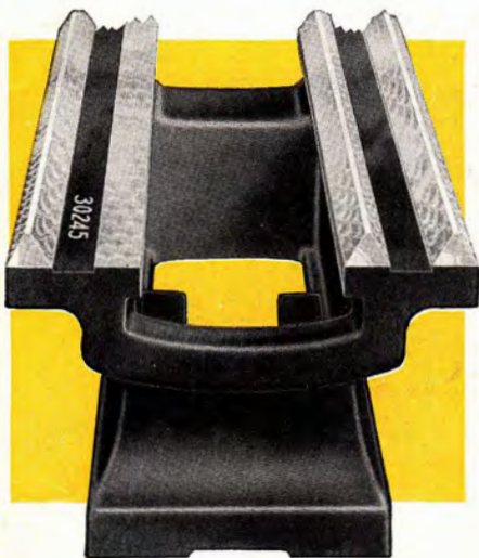
Hand Scraping Tailstock Base to Lathe Bed
