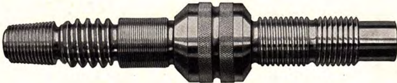
Special Screw Showing Various Types of Threads
