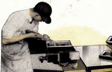
Hand Scraping Tailstock Base to Lathe Bed
