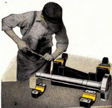
Scraping Bronze Bearings to Receive the Spindle
