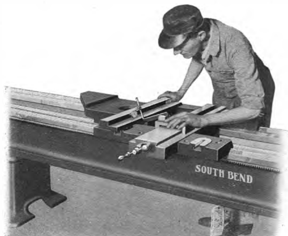
Testing Cross Slide of Saddle with Master Gauge, Using Test Indicator
