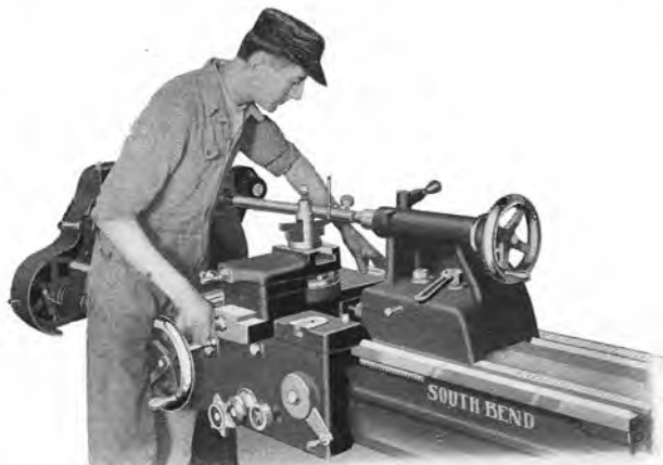
Testing Alignment of Head Stock Spindle and Tail Stock Spindle, Using Test Indicator
