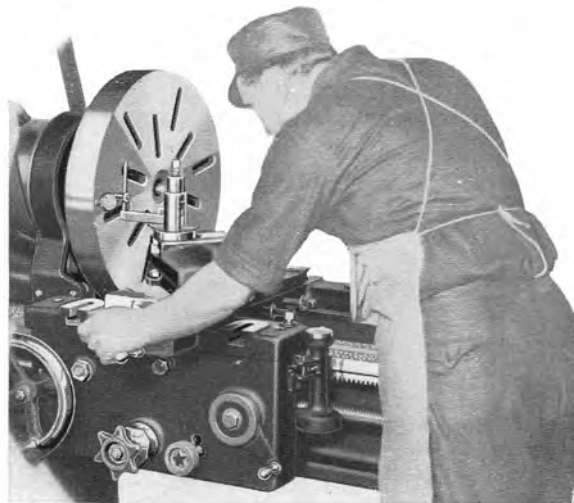
Testing Face Plate, Using Test Indicator
