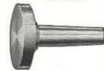
Fig. 187. (Right) Crotch Center for Use in Tailstock of Lathe
