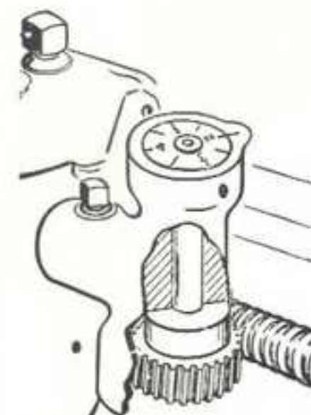
Fig. 237. Thread Dial Indicator Attached to Lathe Carriage
