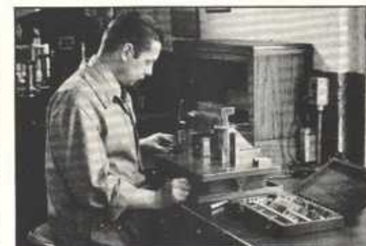
Fig. 364. Toolmaker Locating Holes in Jig Plate with Aid of Surface Plate, Surface Gauge, and Gauge Blocks
