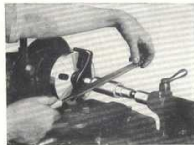
Fig. 265. Filing to Remove Tool Marks
