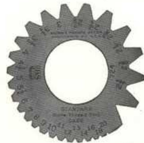
Fig. 216. Standard Screw Thread Tool Gauge for Grinding Thread Cutting Tools
