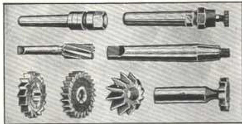
Fig. 299. An Assortment of Milling Cutters and Arbors
