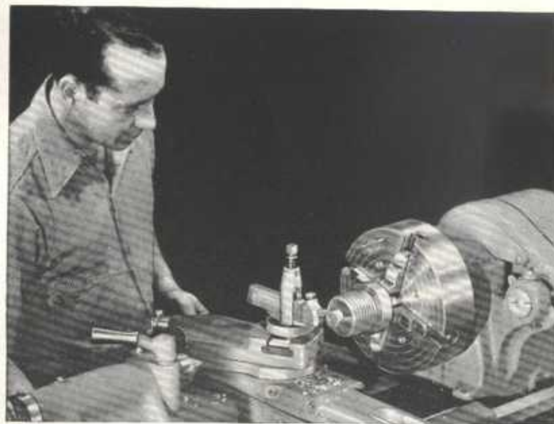
Fig. 204. Cutting Screw Threads in the Lathe
