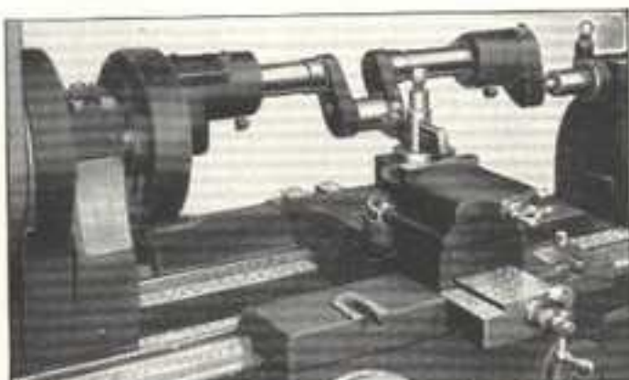
Fig. 335. A Crankshaft Mounted in the Lathe for Machining the Throw Bearing
