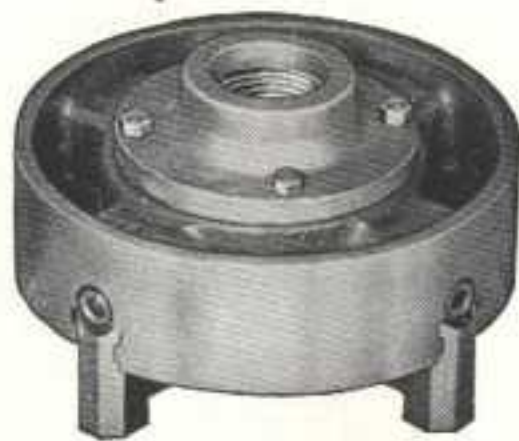
Fig. 348. Chuck with Chuck Plate Attached
