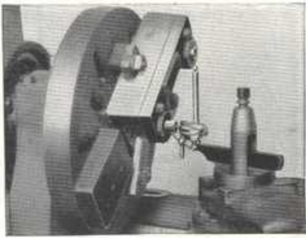
Fig. 264. Locating Work on the Face Plate with a Dial Indicator
