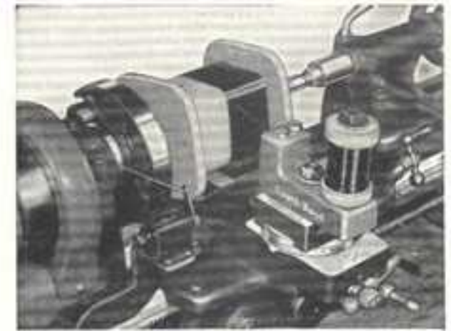
Fig. 273. Winding a Coil
