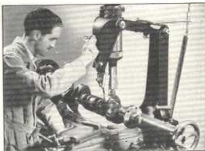
Fig. 336. Truing the Throw Bearings of a Crankshaft by Regrinding in the Lathe
