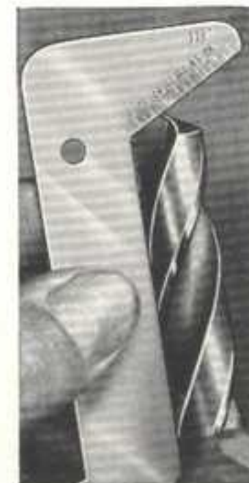
Fig. 200. Drill Grinding Gauge
