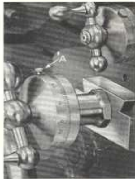
Fig. 226. Micrometer Collar on Cross Feed Screw of Lathe
