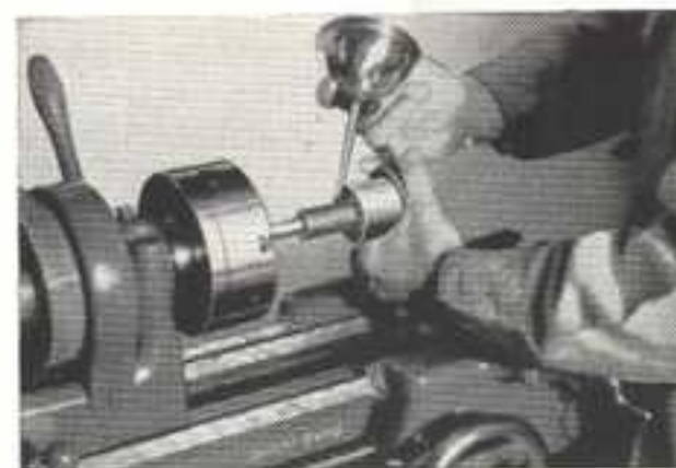
Fig. 267. Lapping the Inside of a Hardened Steel Bushing with Emery Dust and Oil
