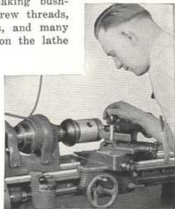
Fig. 329. Turning a Semi-Machined Piston to Size in a 9-in. Lathe
