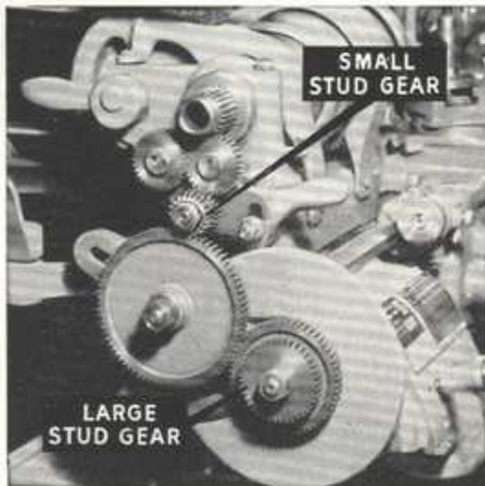
Fig. 211A. Lathe set up for cutting threads 8 to 224 per inch
