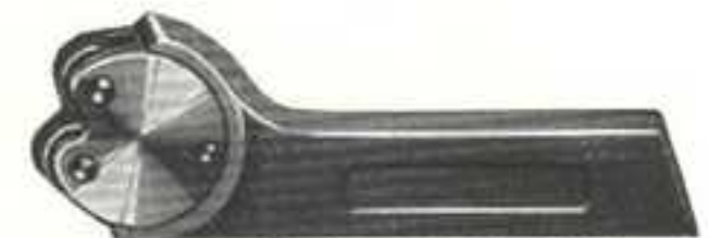
Fig. 258. Knurling Tool for Lathe
