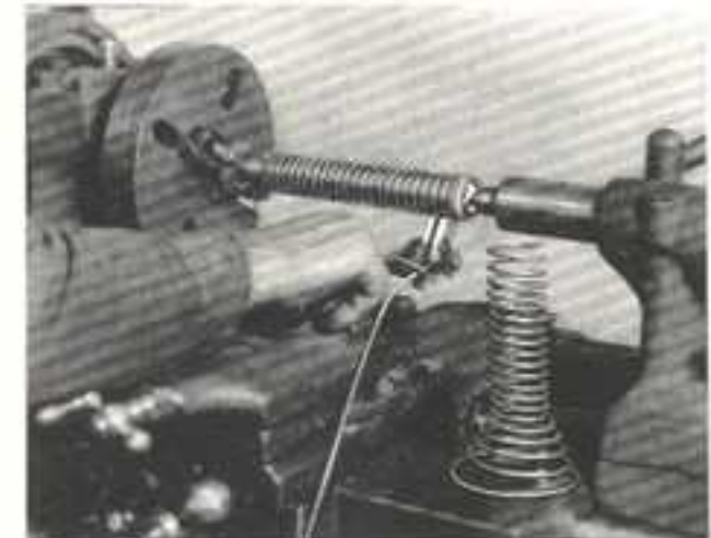
Fig. 274. Winding a Spring
