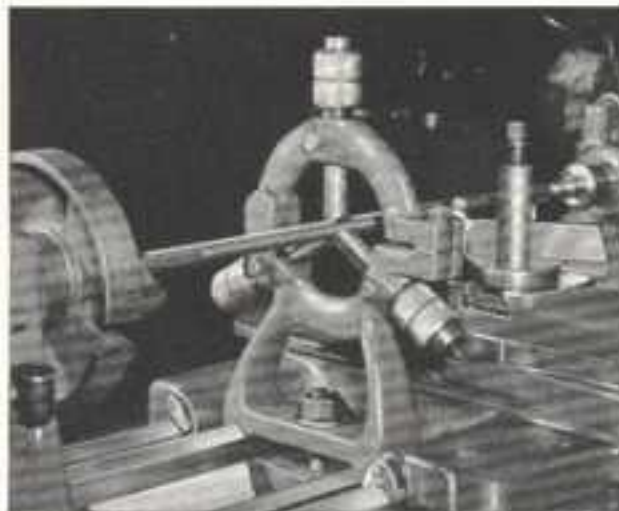
Fig. 280. Telescoping Jaw Steady Rest with Jaws Adjusted to Support Work
