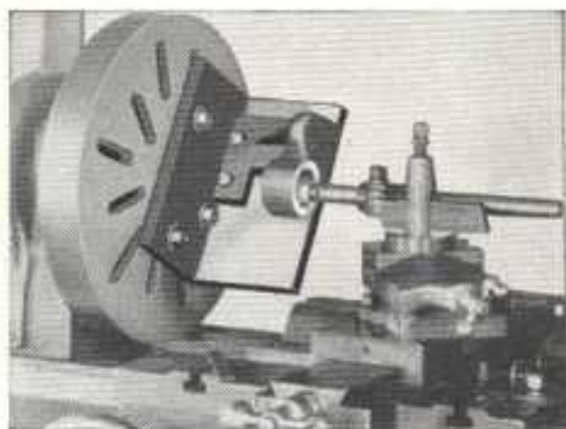
Fig. 262. Boring a Bracket with an Angle Plate Attached to the Face Plate
