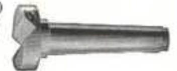
Fig. 187-A. (Left) Drill Pad for Use in Tailstock of Lathe
