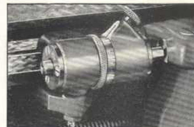
Fig. 310. Micrometer Carriage Stop
