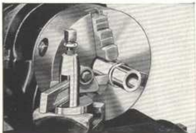
Fig. 328. Making a Replacement Bushing Complete in a 9-in. Lathe
