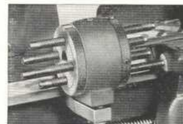
Fig. 311. Four Position Carriage Stop
