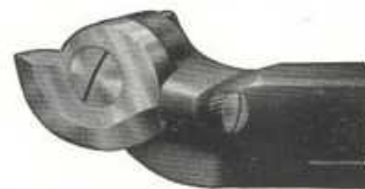
Fig. 215. Formed Thread Cutting Tool, Solid Type
