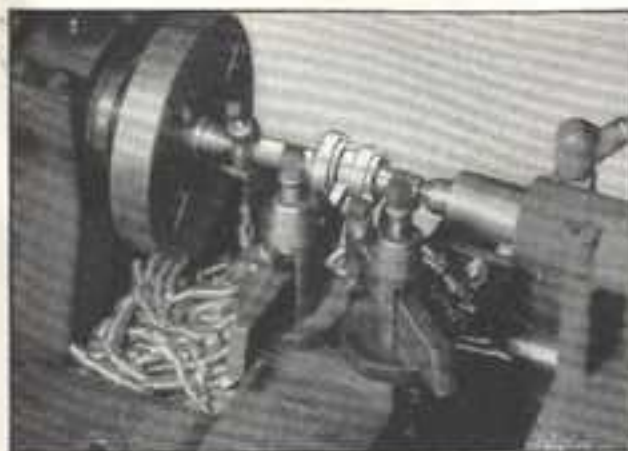
Fig. 295. Two Tools Cutting Simultaneously on a Piece of Work
