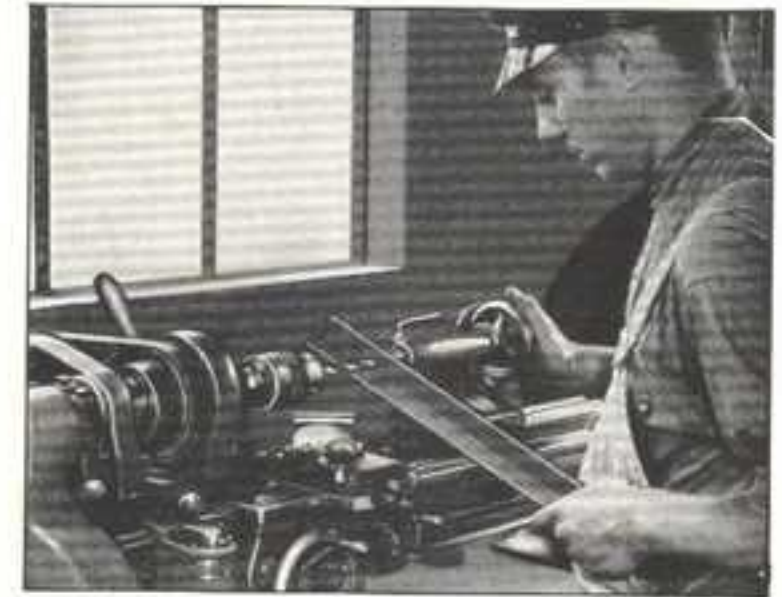
Fig. 186. Using the Lathe as a Drill Press
