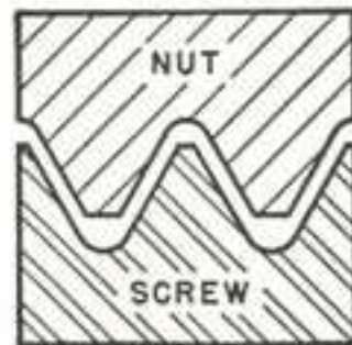
Fig. 208A. Diagram Showing International Screw Thread Form.
