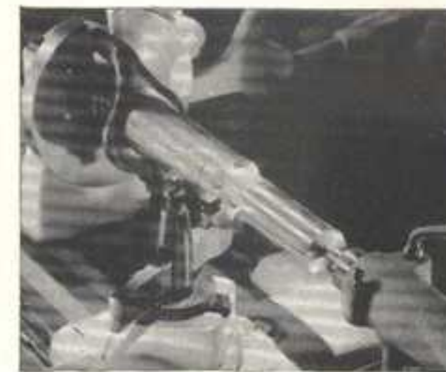
Fig. 356. Taking a Finish Turning Cut Following a Rough Turning Operation
