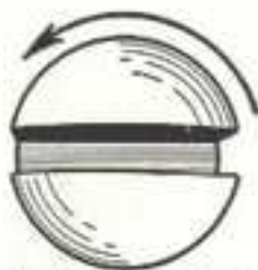
Fig. 235. A Left Hand Screw Advances When Turned Counter-clockwise
