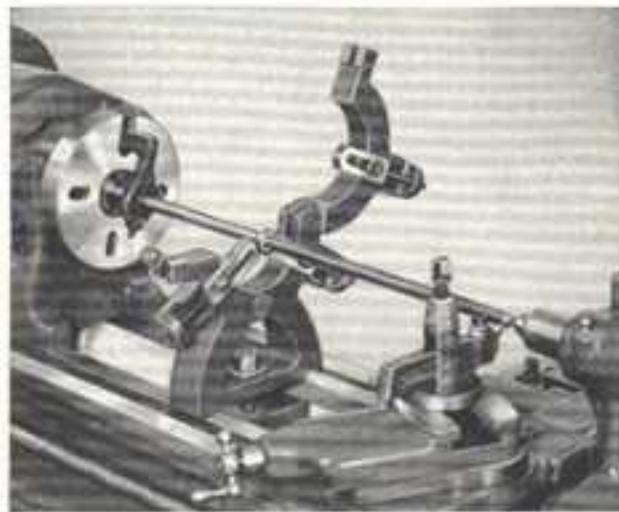
Fig. 279. Steady Rest Mounted on Lathe Bed with Top Open to Receive Work
