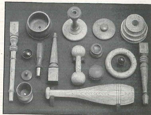
Wood and Fibre Parts Machined in a 9-inch Back-Geared, Screw Cutting Lathe
