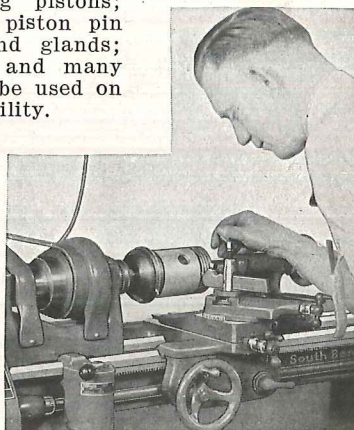
Turning a Semi-Machined Piston to Size in a 9" Lathe
