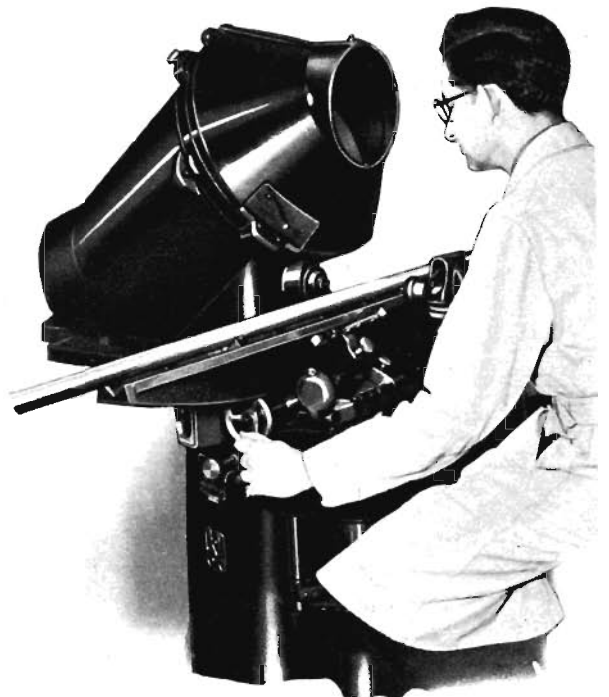
Fig. 1. Inspecting a Screw Thread with an Optical Comparator
