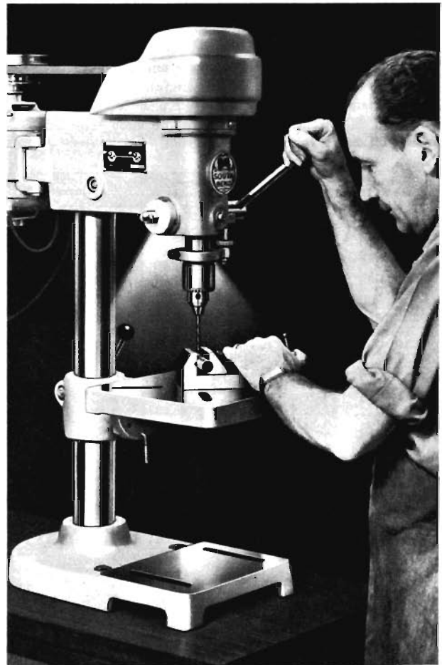
BUILT-IN LIGHT Provides shielded, shadowless illumination on work area. Independent on-off switch is built-in.
