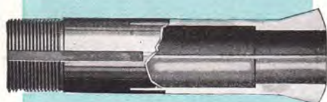
Fig. 53. Cross Section of Collet for 9-inch "Workshop" Precision Lathe.
