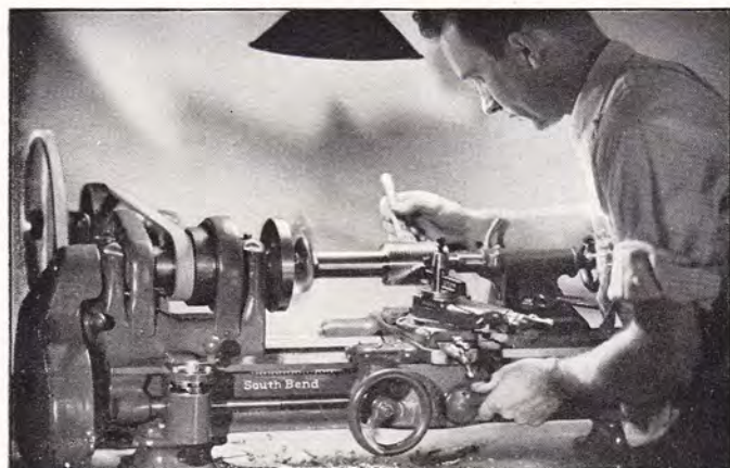
Fig. 33. Cutting a screw thread on a master thread gauge.
