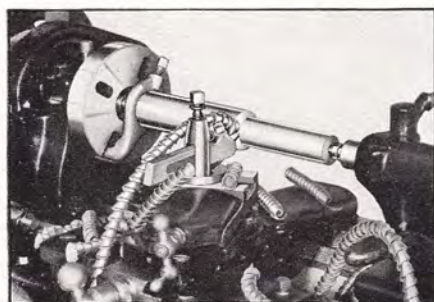
Fig. 34. Taking a heavy roughing cut.
