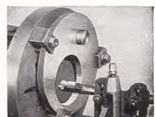
Fig. 91. Boring Work Clamped to Large Face Plate.
