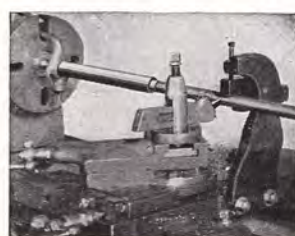
Fig. 89. Using Follower Rest on a Threading Job.
