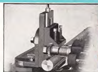
Fig. 71. Milling a Keyway in a Shaft.
