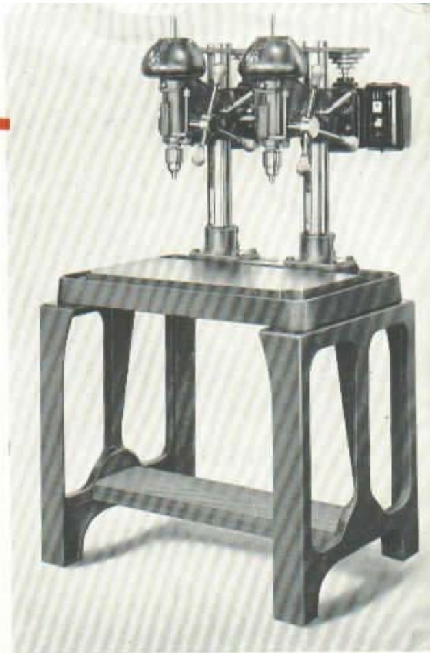
● No. 15 Two-Spindle Drill, Bench Type, on new special "Buffalo" Bench Mounting.
