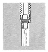
No. 1 or 2 Morse taper and straight shank noses are available in place of or in addition to the standard Jacobs 663 D chuck. The 33 taper bore and locking collar fit the standard 33 taper spindle.
