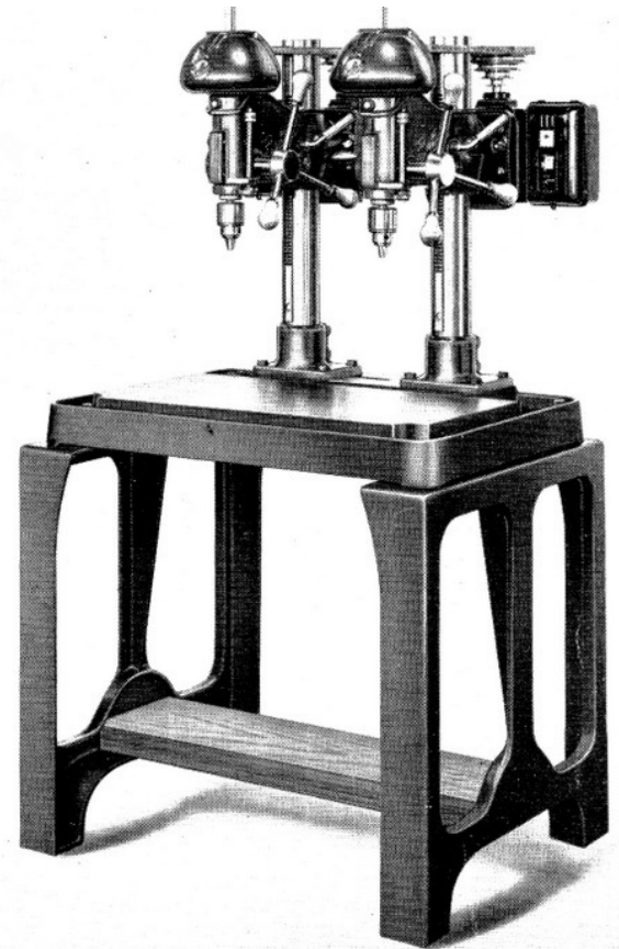
● No. 15 Two-Spindle Drill, Bench Type, on new special "Buffalo" Bench Mounting.
