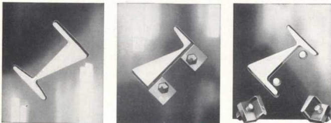
Figure 13. Knives for I-beams and Channels.
