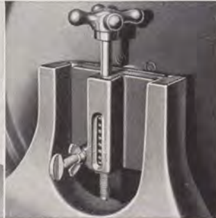
Upper wheel has adjustment for regulating blade tension. Index shows correct tension for various widths of blades.
