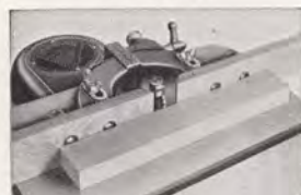
In our fence, both halves are adjustable through one control, and the fence faces—adjustable endwise—permit the cutter opening to be made as small as possible.
