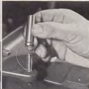
Adjustable leveling stop pin allows table to be accurately returned to level. Can be removed for a 10 degree left tilt.
