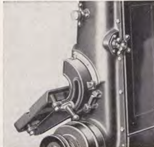
bracket. This is available for use in sanding flat work, to prevent it from being carried along with the belt.
