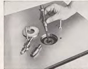
Spindles are readily interchangeable permitting use of wide variety of cutters and stub spindles for cope cuts on sash and doors. Note removable throat disc.
