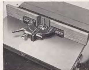
Fully adjustable fence with both halves independent of each other. Adjustable end-wise so opening may be small as possible — a good safety feature.
