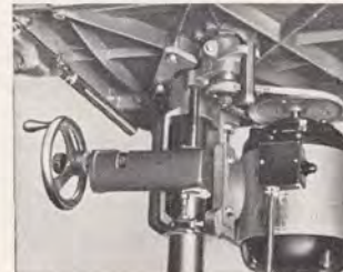
Entire mechanism is a unit assembled and bolted to bottom of table. Nothing to get out of alignment, insures true running.
