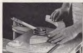
No. 987 Shaper Safety Guard for curved work protects operator from revolving cutters and acts as hold-down.
