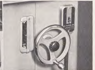
Convenient hand wheel adjust spindle height. Lock knob in center. Adjustable scale plate shows height of spindle. All Controls in one group.
