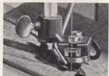
The spring hold-down functions even when the table is tilted; an important feature.
