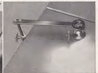
Ring guard not only protects operator from knives but also acts as a hold-down. Does not interfere with shaping operation. A fine accessory.
