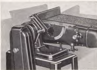
Above. A close-up view of the heavy trunnion that carries the tilting table, showing the swinging stop link and adjustable stop screws. A tilting scale and adjustable pointer are also provided. Right. View from rear, showing adjustable back stop and its
