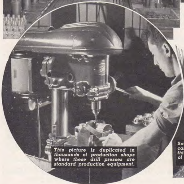
A special set-up of 17" drill press heads in the plant of a large Detroit electrical manufacturer.
