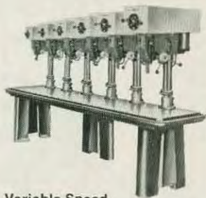
Variable Speed Multiple Spindle Model —Available in 2, 3, 4, 5 or 6 spindles with 1/2" key chuck or No. 2 M.T. spindle, hand or power feed, on both Step Pulley and Variable Speed Models. Can be ordered as cataloged, or custom assembled (either at the factory or in your shop) using any combination of Step Pulley or Variable Speed Heads with any number of spindles from one to a drill press a block long if desired.
