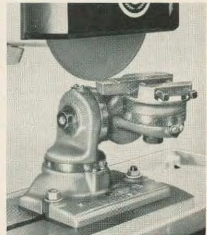
Using a diamond wheel to grind the chip-breaker groove on a tool bit using the 24-902 Univise.
