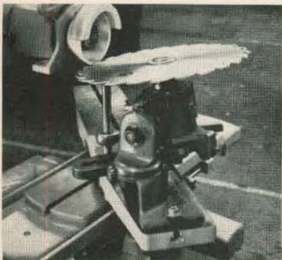
Sharpening a 16" carbide-tipped saw blade using the 24-955 Unihead.
