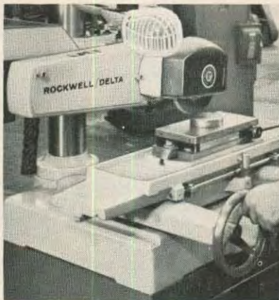
Applying a perfectly true, smooth finish to a part (magnetic chuck not supplied by Rockwell).
