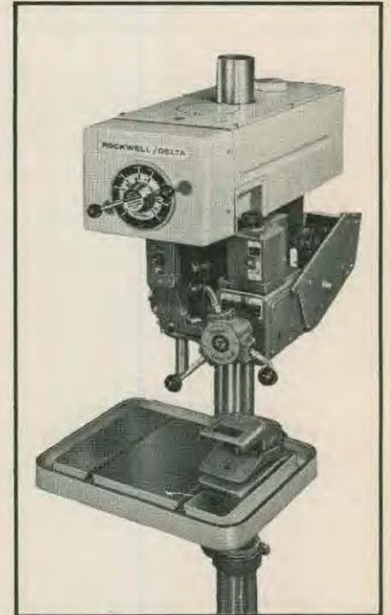
Shown is the Automation and Remote Control Kit with foot switch mounted on a Delta 17" Variable Speed Power Feed Drill Press.
