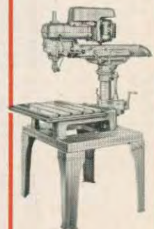
DELTA RAM TYPE RADIAL DRILL PRESS LINE —4 Models Available . . . Hand feed, 6" spindle travel, T-slot production table, key chuck or No. 2 M.T. spindle.
