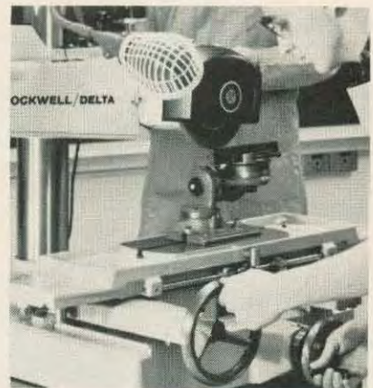
Grinding a new cutting edge on a carbide-tipped tool bit using the 24-902 Univise.
