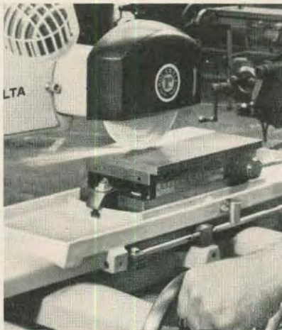
Grinding a precision surface on flat stock (magnetic chuck not sold by Rockwell).
