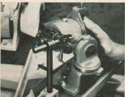
Grinding an angular cutter using the 24-955 Unihead.
