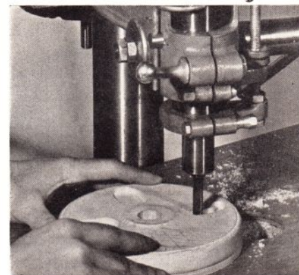
Pattern shops use the router bits in the drill press as shown here for many accurate routing jobs.
