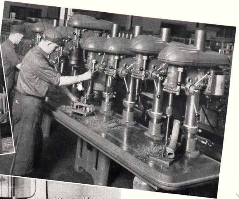
Above — An 8-spindle setup using Delta 17" drill press heads. This is in a machine shop where accuracy is of prime importance.
