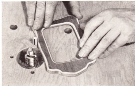
Using the starting or guide pin in shaping an irregular contour against the collars. The work is first held against the pin, then swung slowly into the cutters until against the collars, then swung clear of the pin.
