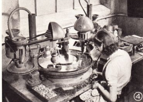
(6) An extra operation obtained by placing a 14" drill on its side on larger machine.
