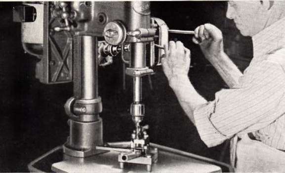
MANUAL FEED OR POWER FEED. No changed parts! Nothing to remove! Machine can be used for either hand or power feed drilling operations.
