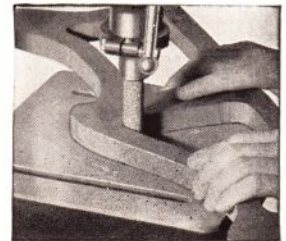
Sanding the edges of curved work with No. 840 sanding drum in No. 974 spindle.
