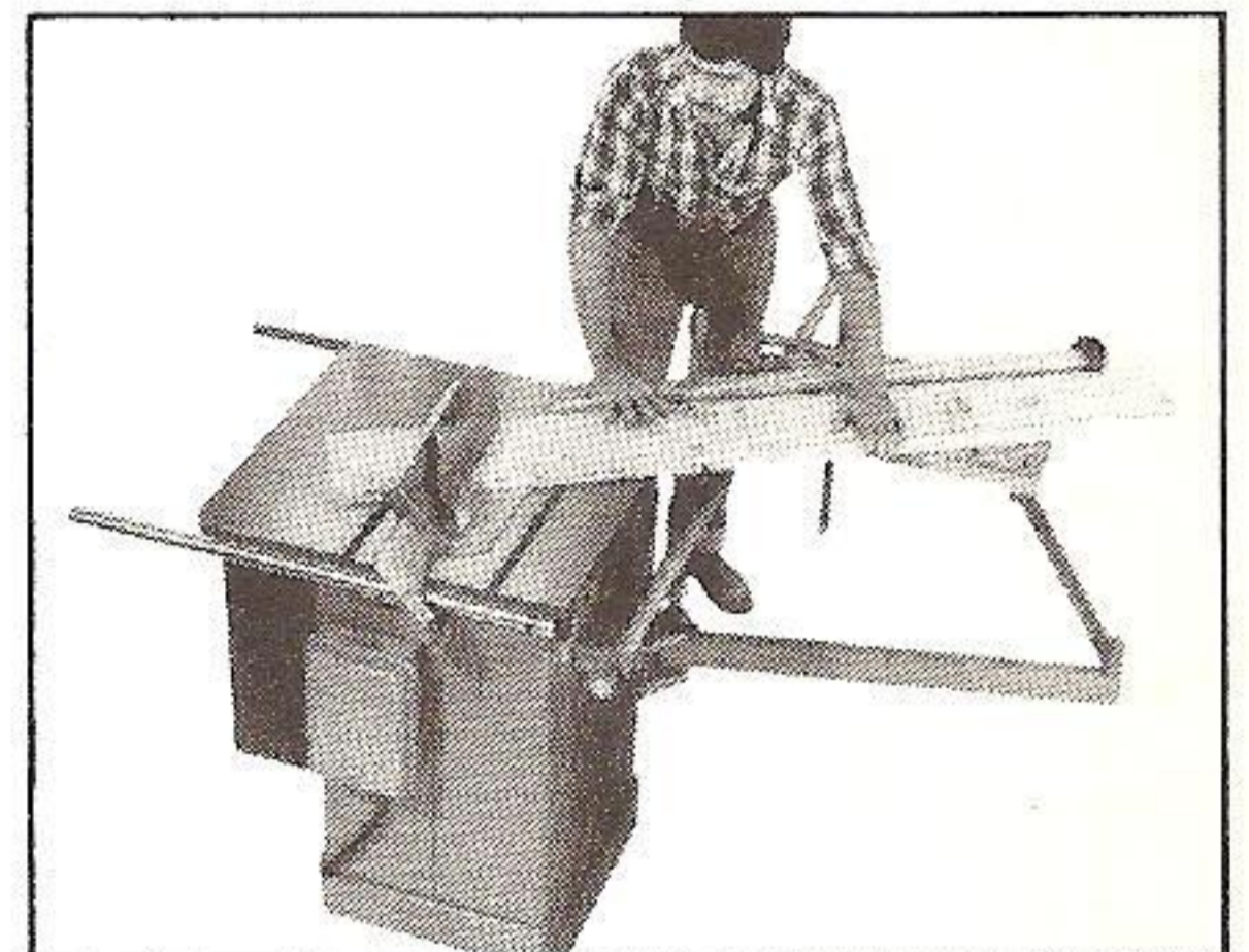
Using mitering fence to cut a compound miter.
