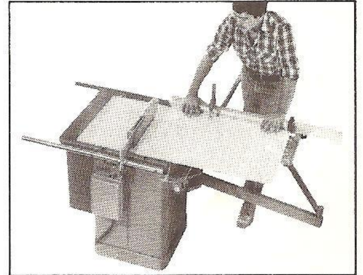
Cutting a panel to a pre-set length.
