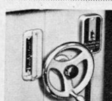
Spindle adjusting hand wheel, starting switch, and spindle height scale grouped for convenient, easy operation.
