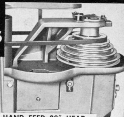
HAND FEED 20" HEAD SHOWN WITH FIVE-STEP GEARED SPINDLE PULLEY
