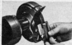
Tool rests adjustable to any angle.
