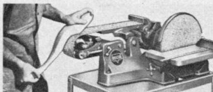
Removable end guard permits inside contour finishing operations on idler drum. Belt tensioning and tracking controls are completely out of the way to facilitate the finishing of extra large, irregular pieces that must be finished on the belt unit.
