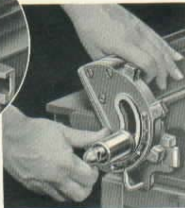
Above, a light pressure of the hand moves the fence across the table when the dual-control handle is slid out to engage the bracket lock and turned to release it. Right, an equally simple motion releases the fence for tilting.
