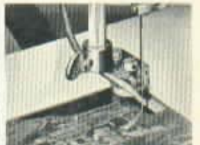
Mortising an engraving—cutting through both wood and metal at the same time.
