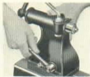
Left, trimming a metal form spur on the No. 930 lathe. Right, no wrench is required to move the tailstock; a handy ball-and-lever locks and unlocks it.
