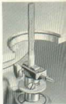
Files, also, are held in the V-jaws of the lower chuck.
