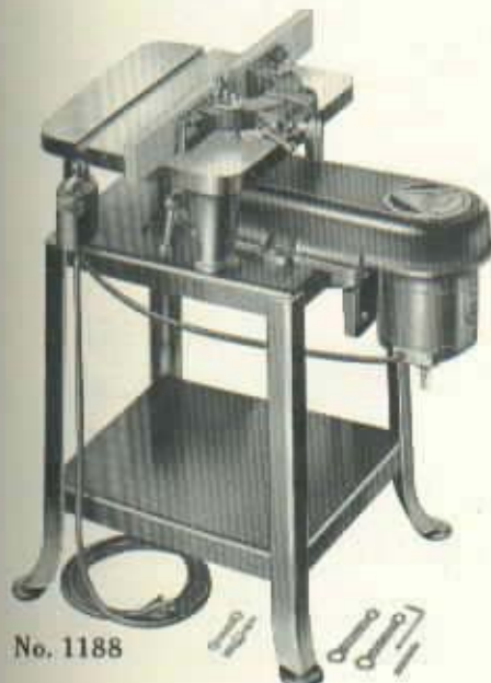
View of the Spindle Adjustment of the shaper. Fast and positive, yet capable of very fine adjustment—and with no backlash.
