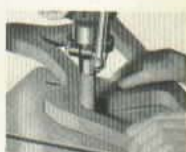
Sanding the edges of curved work with the sanding drum saves hours of tedious labor.
