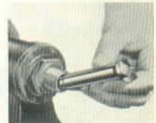
Centers are quickly changed due to the No. 2 Morse taper in head and tailstocks.
