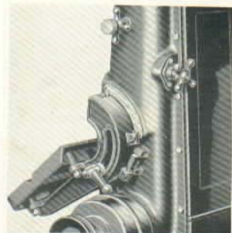
A close-up view of the heavy trunnion that carries the tilting table, showing the swinging stop link and adjustable stop screws. A tilting scale and adjustable pointer, are also provided.
