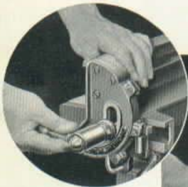
Above, a light pressure of the hand moves the fence across the table when the dual-control handle is slid out to engage the bracket lock and turned to release it. Right, an equally simple motion releases the fence for tilting.
