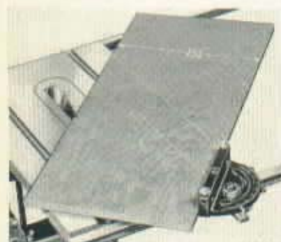
Here is a panel 13 1/2" wide being accurately mitered on the 8" circular saw with front-table extension in place, a job that would be impossible on the ordinary saw with limited room in front of the saw blade.
