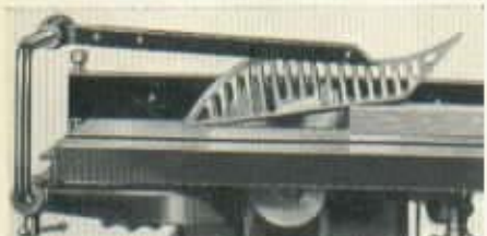
Work entering guard on No. 860 1" saw. This guard, while slightly different in construction details, has all the features of the larger guard.
