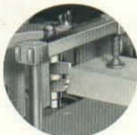
Photo above shows the jig for end-grain shaping from the right side of the machine, showing the stop and pointer on the miter-gage head.
