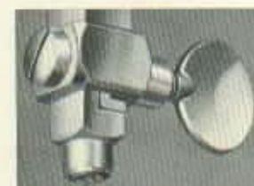
When very fine blades are used constantly, the self-centering chuck jaw is used.
