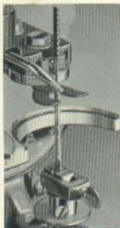
Saber blades are held in the V-jaws of the lower chuck.
