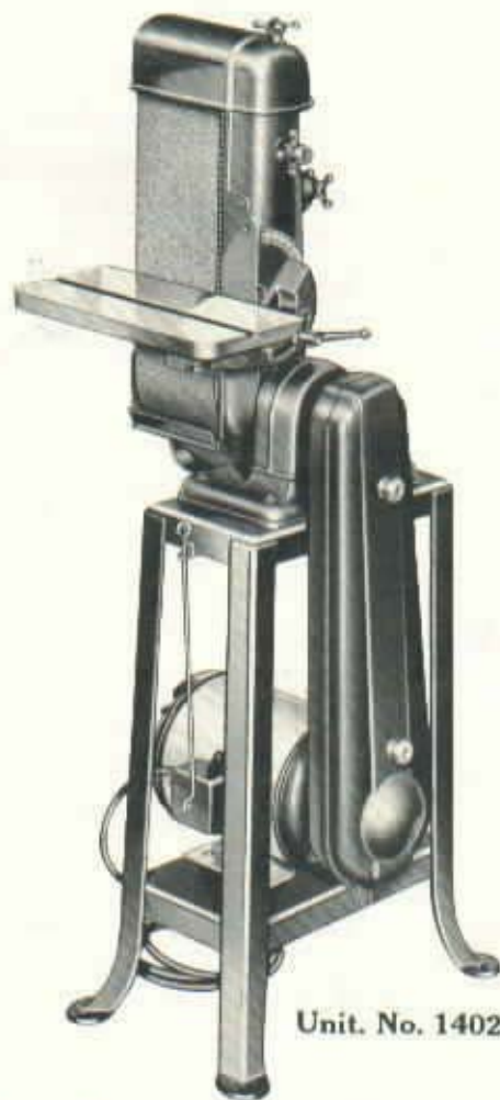
View from rear, showing adjustable back stop and its bracket. This is available for use in sanding flat work, to prevent it from being carried along with the belt.
