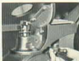
Powerful and convenient hand knob locks the tilting table in the trunnion seats.
