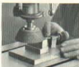
Surface grinding is one of unusual jobs for which this modern tool is adapted.
