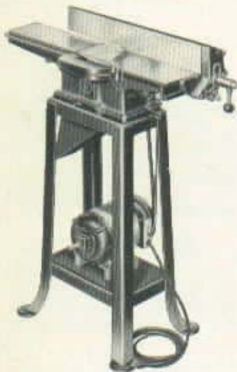
Above, a light pressure of the hand moves the fence across the table when the dual-control handle is slid out to engage the bracket lock and turned to release it. Right, an equally simple motion releases the fence for tilting.
