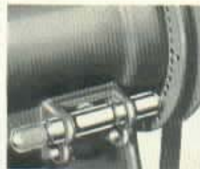
Note double row of index holes in photo at left. At right is shown the graduated tailstock sleeve, with the adjustable pointer.
