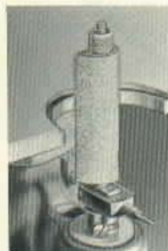
Sanding attachment is held in V-jaws without any change.
