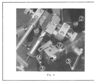
Clamp in position with right hand jaw. Next back off feed screw thimble exposing about  $\frac{5}{8}$  to  $\frac{3}{4}$ " length of thread.
