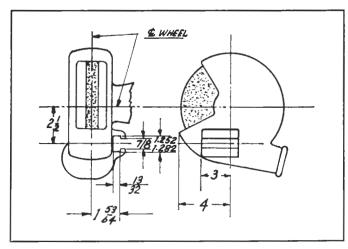
The Improved Drill Grinding Attachment while designed for our grinders may be used on some other types where design permits attachment to be used with an adapter provided mounting dimensions shown above are held. These dimensions establish the relative position of the drill grinding attachment with wheel and guard.
