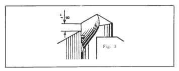
Insert drill with flute engaging locating pin at end of jaw, with cutting lip extending approximately 1/8" beyond end of jaw Figure 3.
