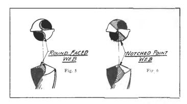
Two common methods of web thinning are shown in illustrations. Figure No. 5 shows the Round Face method, which requires the use of a special ½8" thick wheel with a round face. Figure No. 6 shows the Notch point method, the preferred way and requires no special wheel; the work being done on the regular grinder wheel.
