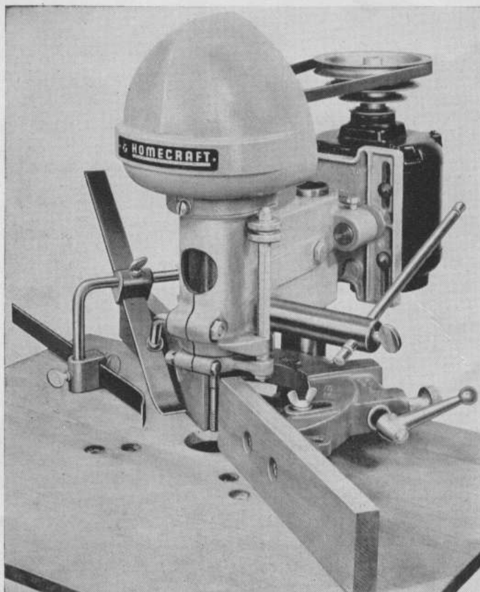
Fig. 7. Drill Press with Shaping Attachments.
