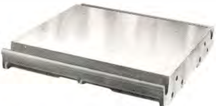
No. 15-155 Production Table , center section, 23 \frac{3}{8} " front to rear x 30" left to right ground work surface with 1 \frac{1}{2} " coolant trough. Use one, two or more center sections for 5- and 6-spindle or larger size tables.
