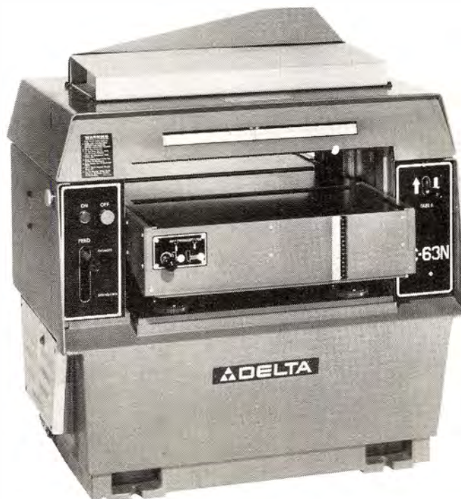
Model No. 22-602 (RC-63N) with Newman "Quiet Cut" Helical Carbide Cutterhead
