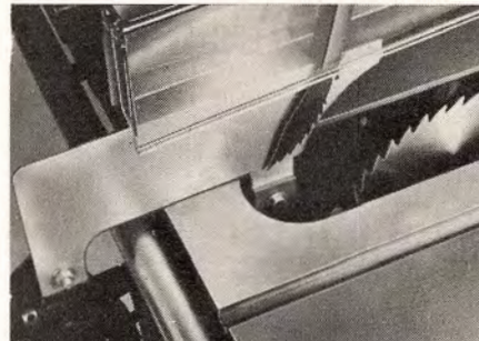
Rigid Splitter Support. Splitter for "clearview" blade guard has a double mounting that provides the rigidity required for accurate cutting. Guard has spring-loaded, anti-kickback fingers.
