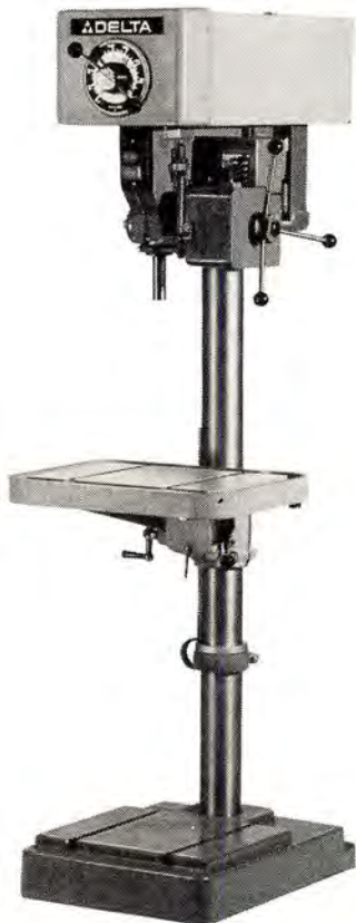
Variable Speed Floor Model shown with production table, No. 2 M.T. spindle and accessory Vari-Rate Mechanical Power Feed. Also available with tilting table.
