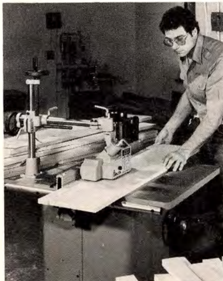
10" UNISAW shown with 34-985 Stock Feeder for fast, repetitive ripping operations.
