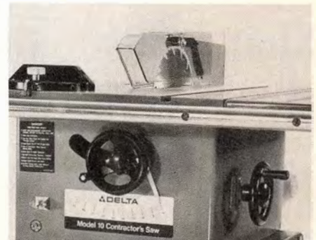
Blade Raising and Tilting Controls. Are located up front for easy, safer operation. Protected on-off switch prevents accidental starts.
