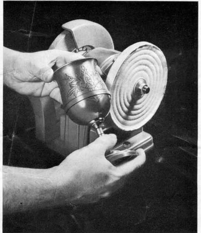
Fig. 5. Buffing gold, silver, sterling and other precious metal cups, etc., to a bright luster.
