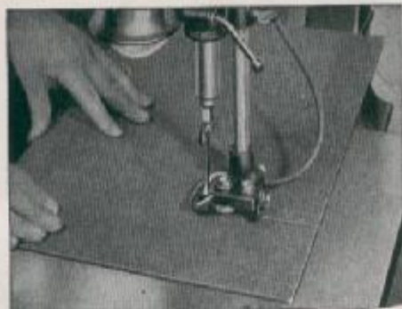
Above, chucks turned 90 deg., and guide post transferred so as to permit cutting from the side
