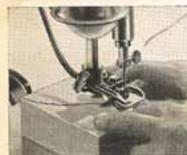
Work up to 1 3/4" thick may be cut on this saw.
