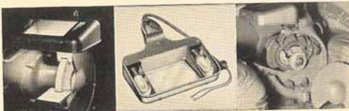
Wheel at 8000 R.P.M. smashed with a bullet. Showing perfect safety of grinder—only danger: bent spark guard!
