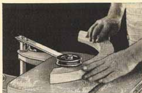
Shaping a curved rail with the No. 987 guard in place. Note how completely the knives are covered.
