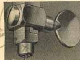
Where very fine blades are used constantly the self-centering chuck jaw is used.
