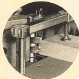
Photo at left shows how the jig is used on a sash operation, insuring absolutely accurate cuts. The photo at the right, below, shows how even a short, narrow block may be shaped safely by the use of the jig.
