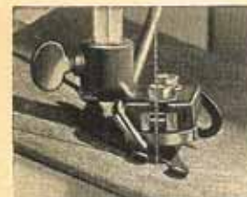
The spring hold-down functions even when the table is tilted; an important feature.
