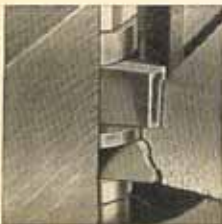
Making a combination rabbet and ogee cut on sash stock, using a spacing collar between cutters.
