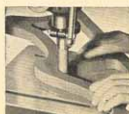
Sanding the edges of carved work with the sanding drum saves hours of tedious labor.
