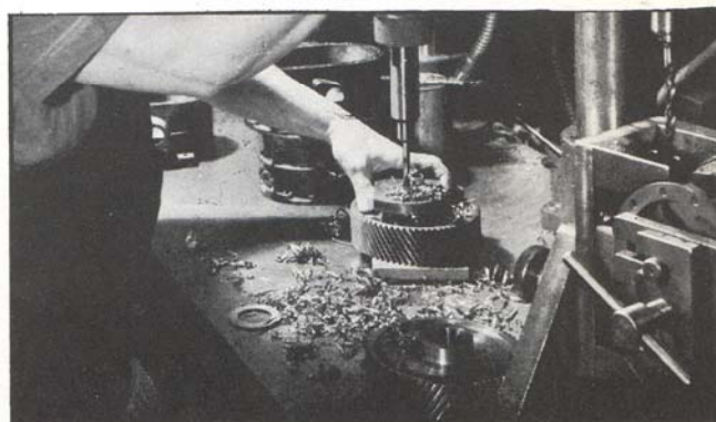
Drilling two \frac{3}{8} " diameter holes with high speed drill for \frac{3}{8} " tap in timing Gear. Heat treated alloy steel Rockwell 40-42 C scale hardness. Slow speed attachment at 200 R.P.M.
