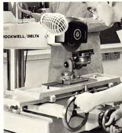
Grinding a new cutting edge on a carbide-tipped tool bit using the 24-902 Univise.
