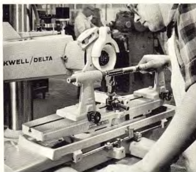
Grinding a reamer.
