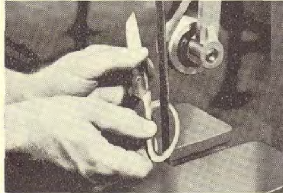
Scissors Manufacturer . . . using narrow band, and without platen, internal grinds rounded edges with ease.
