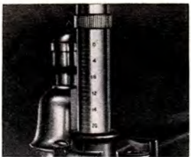
Tension of spring can be adjusted to suit blade, and graduations on tube and adjustment.
