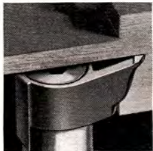
Above is shown special sash cutter D-128, with stub spindle, making cope cut on sash rail.
