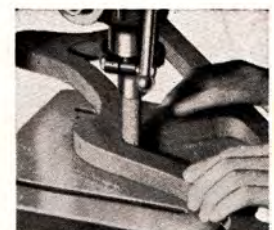
Sanding the edges of carved work with the sanding drum saves hours of tedious labor.
