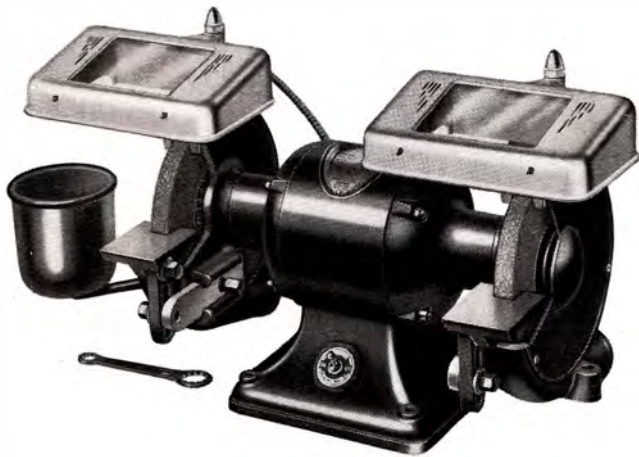
Wheels are so set that long work can be passed over wheels without interference.
