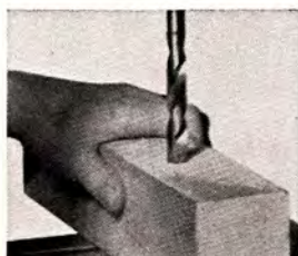
Boring in wood with spur bits is practical because of the standard high speed.
