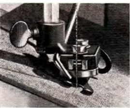
The spring hold-down functions even when the table is tilted; an important feature.
