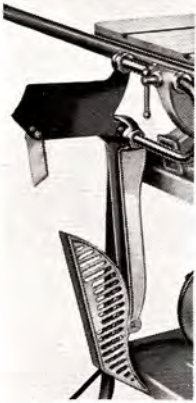
These guards may be swung completely back and out of the way in a second's time, and as quickly swung back when needed. They need never be removed for any reason.
