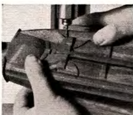
Using small carving bits for carving in the round saves hours of patient labor for the carver.
