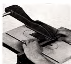
The guard is made of heavy cast iron, completely closed so that no particles can be thrown out.
