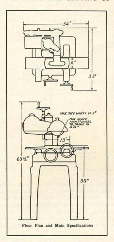
Machine should be carefully uncrated and cleaned of all packing grease. In case there is no crane for handling available, the machine should be laid on the belt guard side with proper blocking under the side of the base casting to prevent breakage of the weaker castings.
