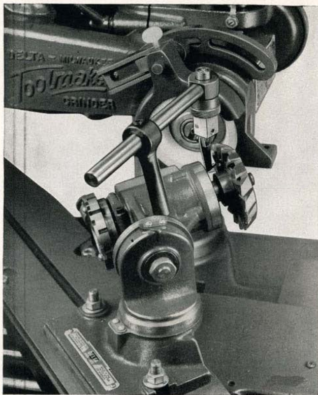
Grinding an (Dovetail) Angular Cutter
