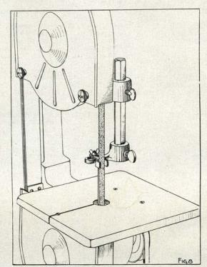
dullness of the teeth or absence of sufficient set or clearance, (5) excessive tightening of the blade on the wheels, (6) top guide set too high above the work being cut and, (7) using a blade with a lumpy or improperly finished braze or weld.
