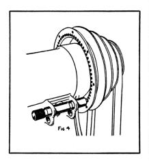
et, so that it will align with the inner row of 60 holes, and the end of the pin is inserted into one of the holes in the pulley rim. The flute is then cut in the work by means of the portable router or flexible shaft, (Fig. 5) then the index pin is withdrawn from the hole, the pulley turned forward, counting the holes as this is done, and the index pin re-inserted into the tenth hole.
