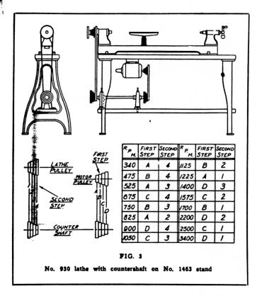
ment speeds ranging from 340 to 3400 R. P. M. can be obtained. The chart (Fig. 3) shows the various speeds obtainable through the use of different pulley arrangements. The slower speeds are especially useful for large faceplate work to be done on the outer end of the spindle in connection with the floorstand for the tool supports (No. 697 shown in Fig. 6).
