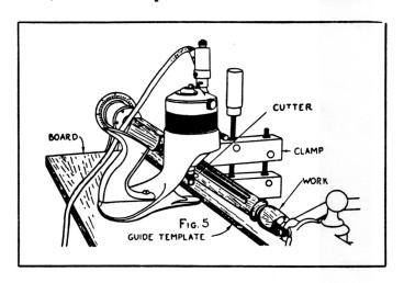
After the second flute is cut, the pulley is turned forward another ten holes, the third flute is cut, and so on until all the flutes have been cut. Simply dividing the number of holes in the row by the number of flutes to be cut will give the number of holes that must be taken each time—and it will be noted that 8 and 60 provide a very large number of possible divisions.
