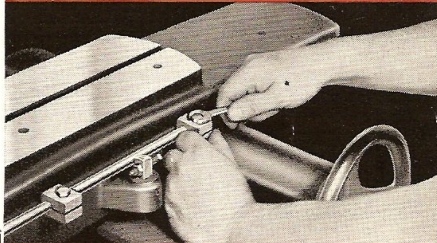
Readily accessible clamp blocks and set screw allow accurate setting of longitudinal table travel. Maximum travel is 13½". Removal of block holding set screws allows table to be completely removed.
