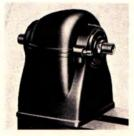
Safety Headstock completely en-closes pulley and belt from front and top of lathe. Belt drive can be taken from either the bottom or the rear — an added convenience.
