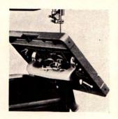
The handy to get at blade guides and blade supports are individually adjustable. You can set one without affecting without affecting the other. Notice also the adjust-able table stop that enables you to return the table to exact level after tilt-ing.
