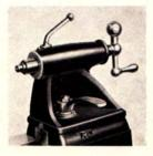
Graduated Tailstock Sleeve operated with large erated with large bail crank handle and locked in place with con-venient ball end lever. Sleeve ma-chined for No. 2 Morse Taper cen-ters. Centers self-ejecting.
