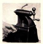
Substantial, finegrained cast iron tailstock, with sub-base and provi-sion for set-over of tailstock for center alignment and taper turning. Tailstock locks to bed with wrench conveniently located at front.
