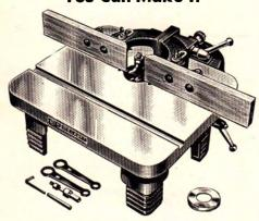
Designed for high-speed, light duty production work. Cuts smoothly and rapidly at all possible angles to the grain of wood. Four features exclusive in this price range (1) both sides of fence adjustable through a single control (2) Interchangeable spindles permit use of wide variety of cutters (3) spindle height adjustment under front of table makes accurate height adjustment easy. Locks quickly in place. (4) Closely spaced bearings eliminate chatter.
