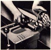
Improved fence mounted with worm gear tilt adjustment and positive lock. Fence locks in position anywhere across the table. Rigid construction prevents twisting or warping.
