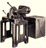
The large amount of abrasive material and metal dust produced by the Cut-Off Machine is thrown into the air and must be collected to protect the operator and the machines. The Dust Collector is perfectly adapted for this use, catching the metal dust and abrasive material in the tray and filter of the unit.
