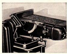
View showing No. 1403 adjustable back stop and its bracket. This is available for use in sanding flat work, to prevent the work from being carried along with the belt.
