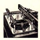
Sliding Shaping Jig — Shaping of short and narrow pieces is now a safe, accurate operation with this sliding shaper jig. Hands never come close to cutter and work cannot slip. Wt. 19 lbs.
