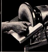
All kinds of sanding can be done quickly and easily—free hand curved sanding, sanding with jigs, angle sanding, miter sanding, etc.
