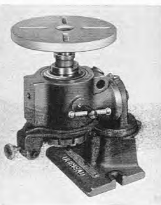
Unihead with Delta Cat. No. 937 6" face plate in place. Useful for mounting jigs and fixtures
