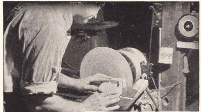
The Abrasive Disk Finishing Machine is used in hundreds of pattern shops.
