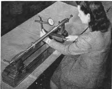
Precision Testing Photograph shows operator checking the taper of a grinder spindle for runout.
