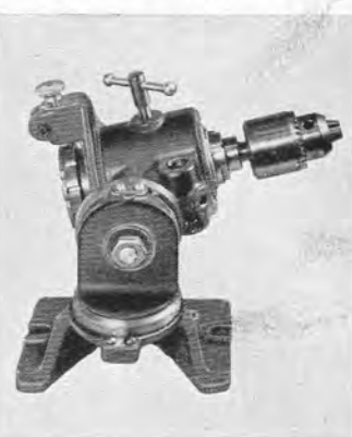
Photo showing Delta Unihead with 1/2" No. 6A Jacobs chuck in place
